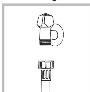
1. Connect the supply pipe by screwing it to a cold water tap using a  $\frac{3}{4}$  gas threaded connection (see figure).
